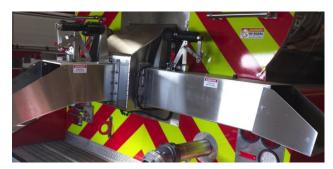
1070-34 electric stainless steel dump valves with a fixed length, and include a flip down extension.
