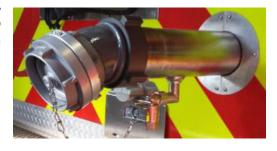
Internal tank will have a fast fill diffuser installed as part of the valve.
